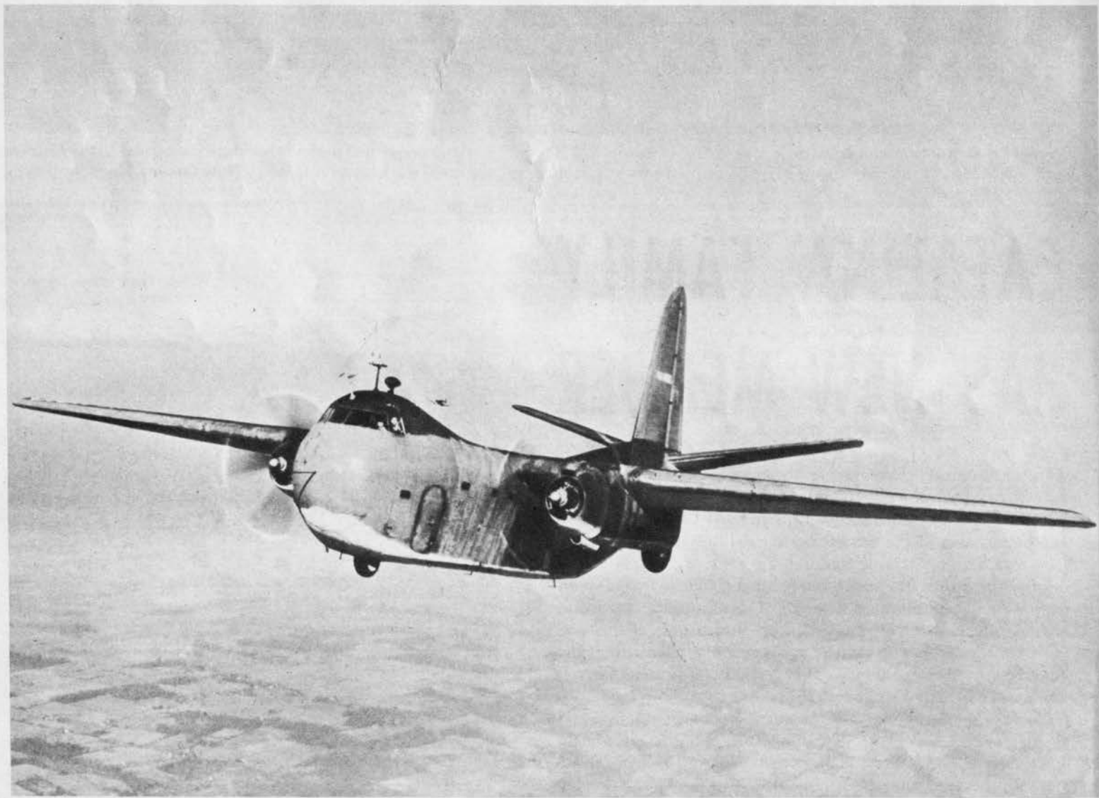
RB-1's wing is bar-straight but the tailplane has a very pronounced dihedral. The fuselage consists essentially of a long and squarish cargo
